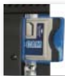
Ingresso COMMON INTERFACE
